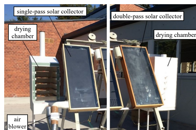
Fig. 2. Complete installation of solar drying system.
